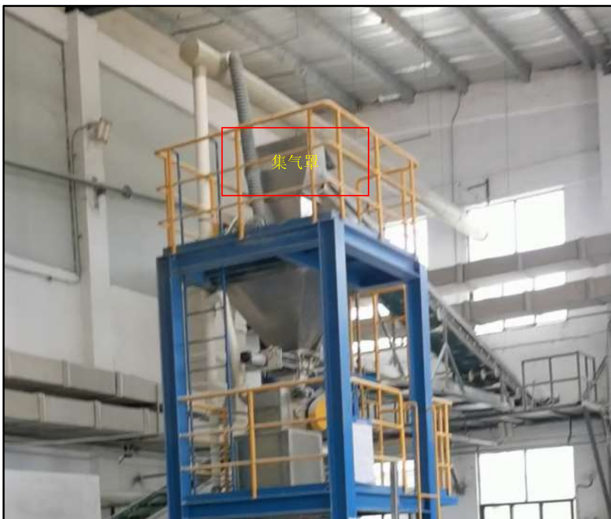
图8.3-1 软片破碎粉尘拟设集气罩示意图
